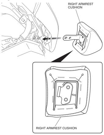
9. Install the plate nut as shown.
